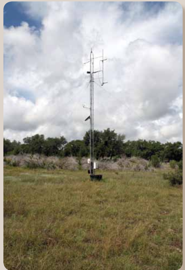
Figure 1. Evapotranspiration station in the treatment watershed at site TWS ET (U.S. Geological Survey station 295102098283200 Honey Creek treatment evapotranspiration near Spring Branch, Texas), Honey Creek State Natural Area, Comal County, Tex., July 23, 2010.
